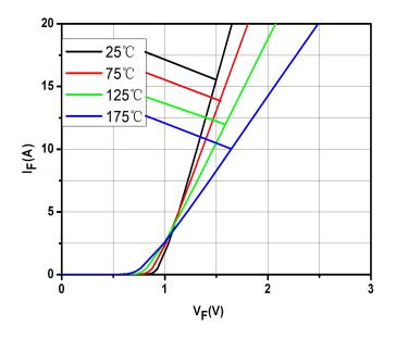
Fig.1-Typical Forward Voltage Characteristics
