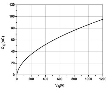
Fig.6-Total Capacitance Charge vs. Reverse Voltage
