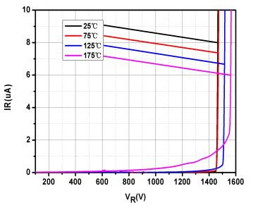
**Fig.2-Typical Reverse Characteristics**
