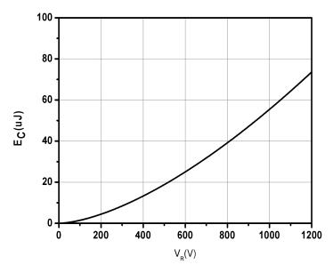
Fig.7-Capacitance Stored Energy
